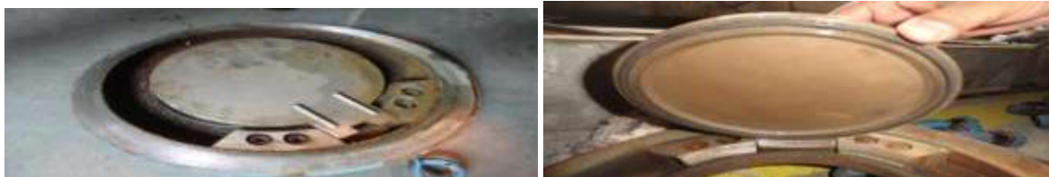
Fig. 21 Suction NRV without “o” ring and suction NRV with “o” ring.
