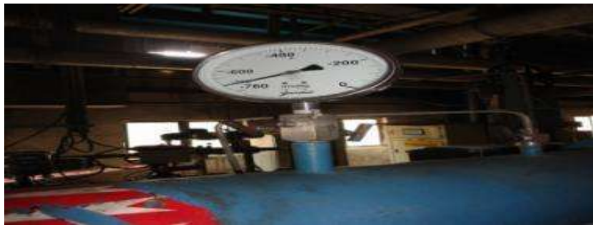
Fig.5 Suction pressure measured during shutoff head
